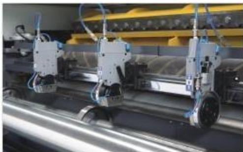
Slitting knife is used for cutting.
