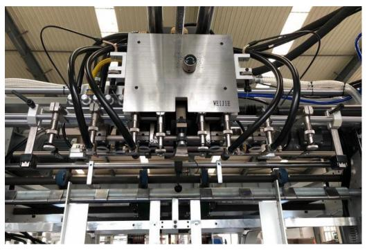
4. Sensing and compensation and alignment device uses several groups of sensors to sense the relative position of the running corrugated board so that two servo motors at left and right side of the top paper can drive independently to align top paper with corrugated paper with high accuracy and high speed.
