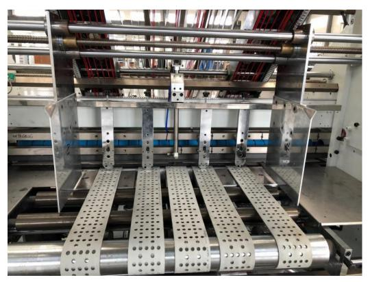
9. When order is changed, the operator can change the order easily by input the paper size and touching one key, all the adjustment can be finished. It also can control with hand wheel separately.
